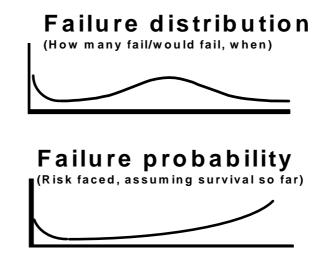
Figure 3. Failure Distributions vs. Underlying Probability Patterns
