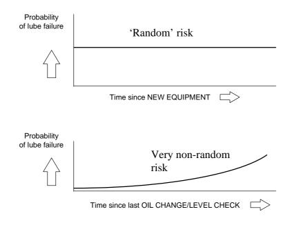
Figure 4. 'Random' is relative: lubrication failures example
