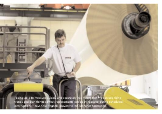
Olle Regnell is a preventive maintenance technician at the Skoghall Mill, a company within the StoraEnso group. In 1993, the company installed extensive on-line equipment for the shock pulse measuring of bearings on Board Machine No. 7 (BM 7). Thanks to this investment, today they can measure, with a focus on wrapping, drying and pressing quantities in the board machine, 1,050 items of stock every 24 hours. Earlier it took between four and six weeks to do the same job!
